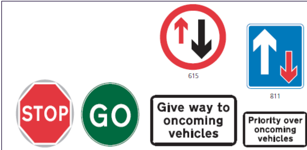
Figure 1.6.1-5: Manually operated stop/go signs and priority signs
